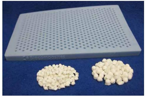
Figure 5: Photograph showing Stimulan Bead Set. The blue plate is a sterile, silicone mat that can make 3 different sized beads (3, 4.8, and 6mm). In this series we primarily used 3 and 4.8mm beads to increase overall surface area and allow for faster dissolution of Calcium Sulfate. The beads shown here are from a 10cc batch of Stimulan. The smaller beads are 3mm diameter beads. The larger beads are 4.8mm diameter beads.
